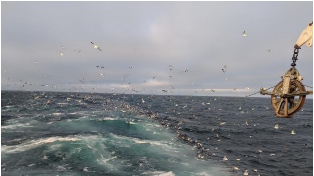
Figure 2. The view looking astern of a hake catcher-processor vessel, showing seabirds flying in the vicinity of the third and fourth wires. These cables transmit data from a net sonar device and a live video feed near the codend of the net. Photo courtesy of A-SHOP program.
