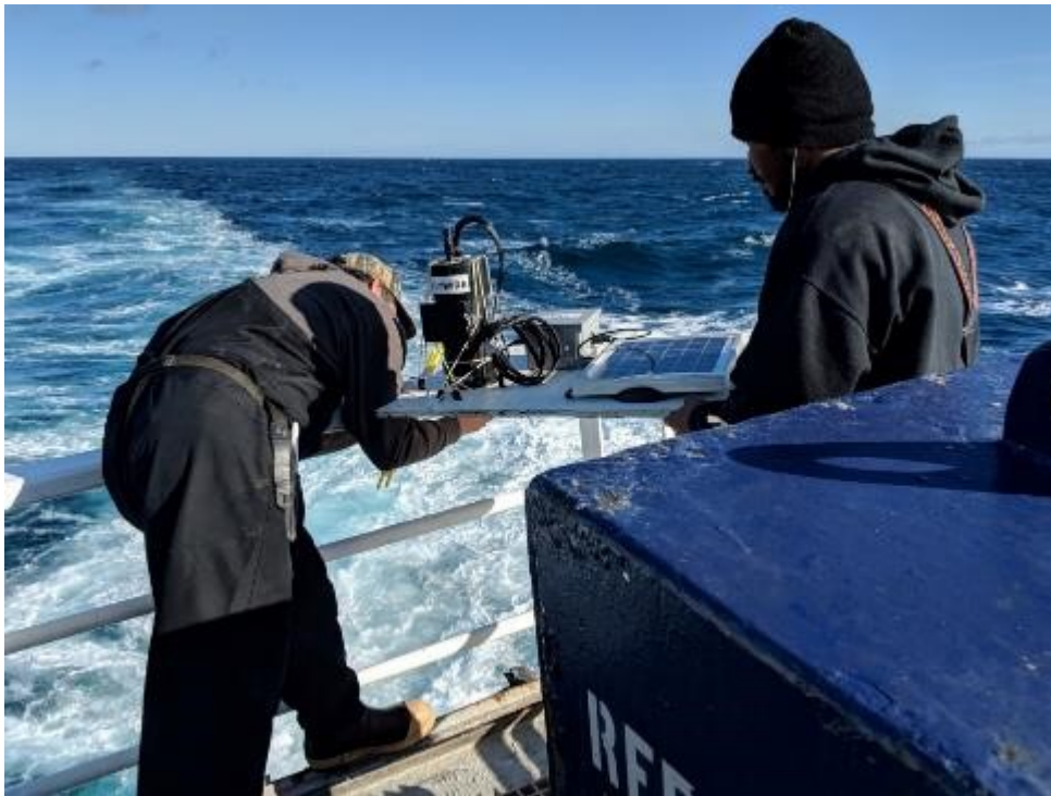
Figure 4. An electronic video monitoring system during operational feasibility testing on the F/V Seattle Enterprise during the Fall 2018 hake season. Photo by Amanda Gladics
